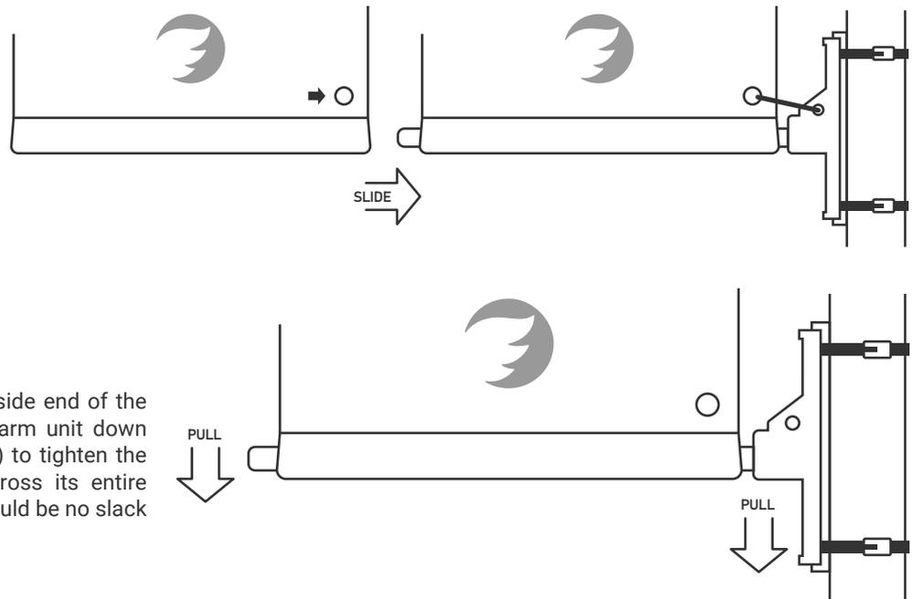
While you pull down on the outside end of the fiberglass rod, slide the entire arm unit down enough (rocking it, if necessary) to tighten the banner so it is evenly taut across its entire surface. **IMPORTANT:** There should be no slack on the INSIDE of the banner.
