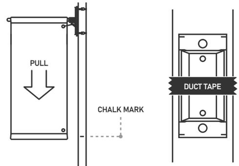
6. - Next, slide the BOTTOM sleeve of the banner onto the arm (make sure grommet is toward pole). Slide the Arm Unit onto the bottom mounting plate with the support wings of the rod socket pointing UP. Insert the two self-locking bolts through the adjustment slots in the Arm Casting and thread them LOOSELY into the Base Casting.
