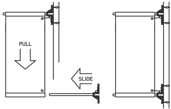
5. - . The second banding strap should now be installed around the pole and over the bottom banding guides. Hand tighten the band, drawing the bottom of the arm unit snugly to the pole. The banner should be evenly taught across its surface without any wrinkles or stretch marks. Once you have adjusted the bottom bracket up or down to achieve the desired look, then, hand tighten both pieces of strapping securely.
