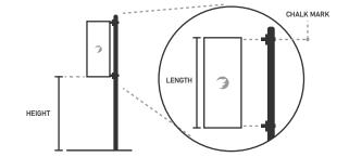
2. - Mount the TOP Bracket to the pole with two of the banding straps (duct tape holds the unit in place while you strap it).
